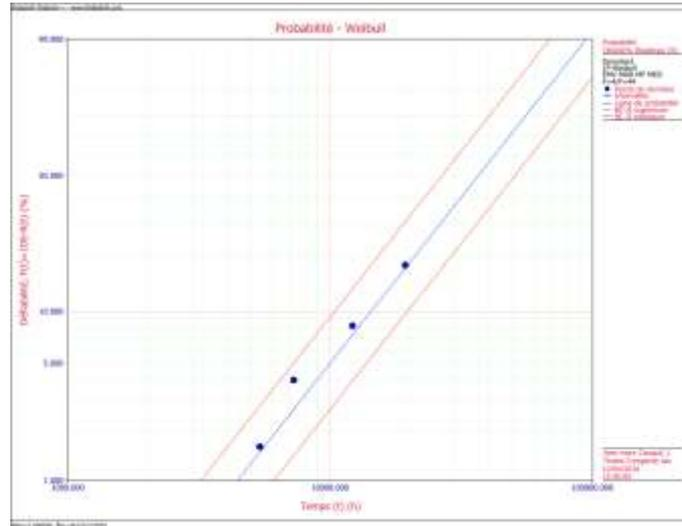
Figure 6: graph of Weibull law for the failure mode: bearing damage in A20 test.
