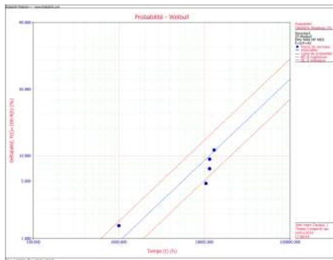
Figure 8: graph of Weibull law for the failure mode : process defect in A20 test.
