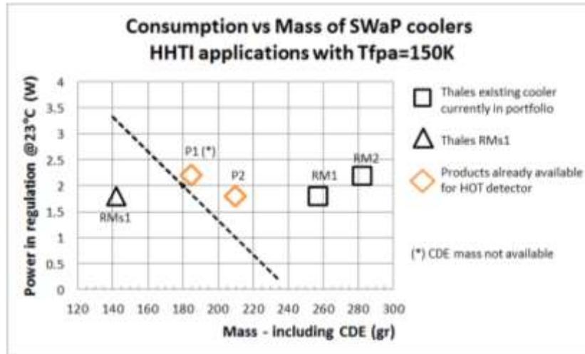
Figure 19: Trade-off between Weight and Power driven by battery specific power at HHTI level. The bold line is based on a 2WDC consumption for 180gr at 150K (Initial target). The slope of the bold line shows an example of specific power. The sensitivity expressed by the bold line slope is based on following assumptions: a specific power of 200W/Kg (Lithium-Ion Battery) and autonomy of 4 hours. The sensitivity of the system is typically of 30gr/W [7]
