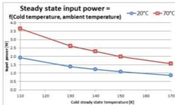
Figure 6: Steady state input power as a function of cold temperature and ambient temperature
