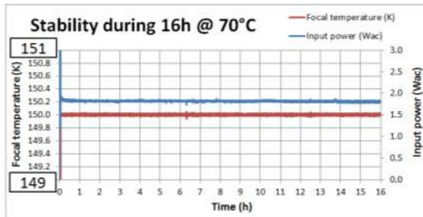
Figure 10: Temperature and input power stability during 16 hours at 70°C. the full scale is +/-1 Kelvin for focal temperature and 0-3W for input power.
