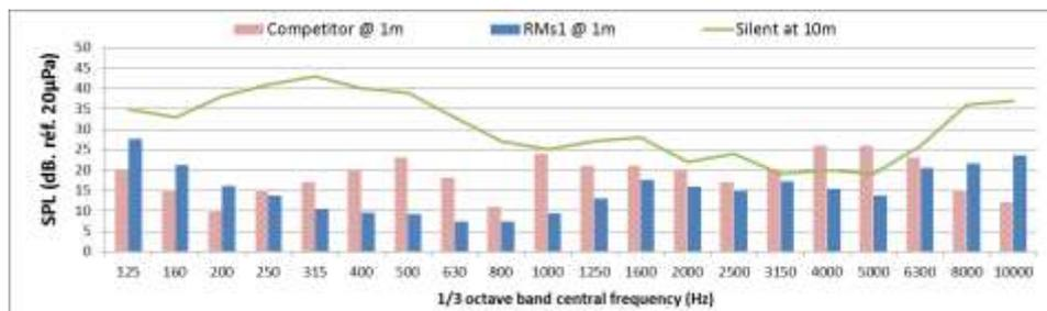
Figure 14: Comparison of RMs1 acoustic noise with competitor
