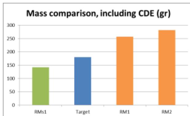
Figure 18: Weight comparison of RMs1 with RM1 and RM2. The mass includes driver electronics weight
