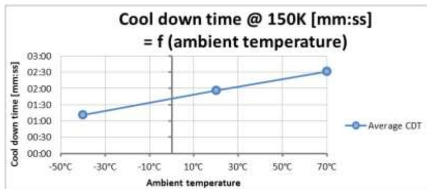
Figure 4: Cool down time as a function of ambient temperature
