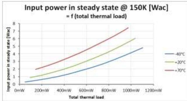
Figure 8: Steady state input power at 150K in function of ambient temperature and total cooling power
