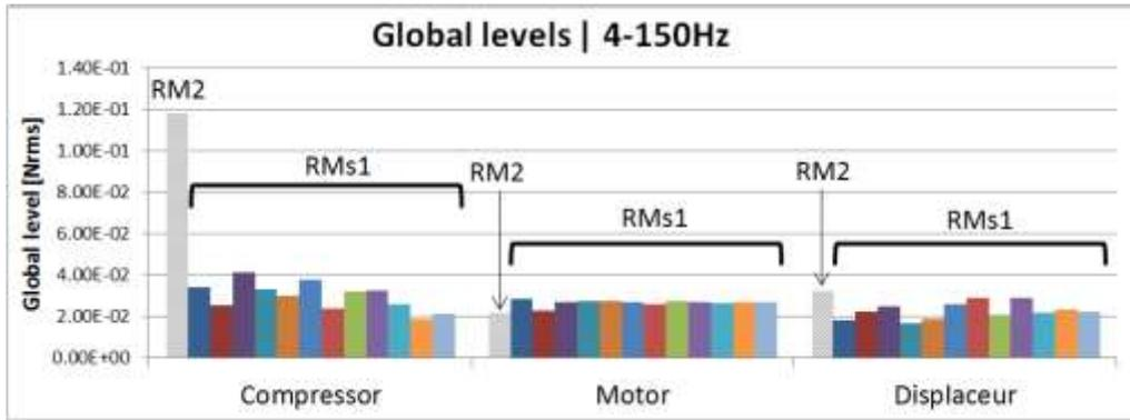
Figure 12: RMs1 global induced vibrations levels and comparison with RM2
