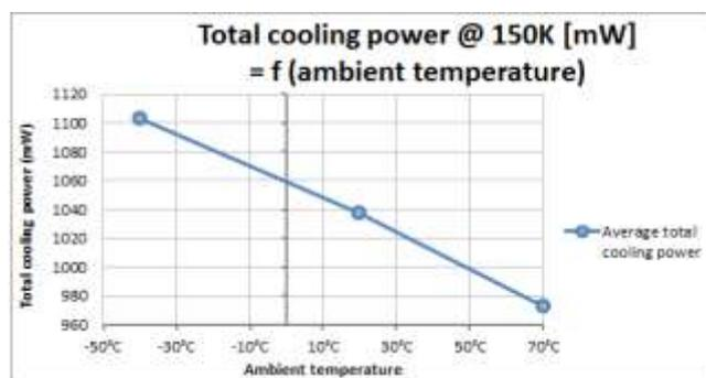
Figure 9: RMs1 total cooling power at 150K in function of ambient temperature
