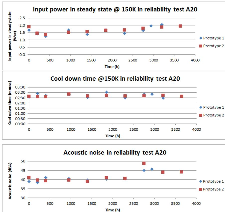
Figure 20: Lifetime test intermediate checks
