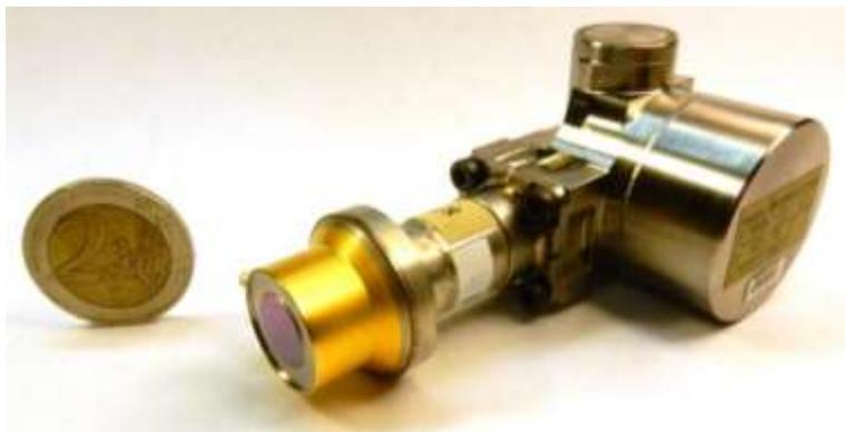
Figure 3: RMs1 prototypes, integrated in a dewar thermal mock-up
