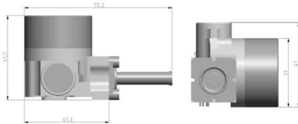
Figure 1: Overall dimensions of RMs1 integrated in common cold finger
