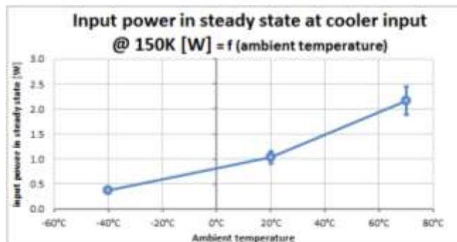
Figure 7: Steady state input power at 150K as a function of ambient temperature
