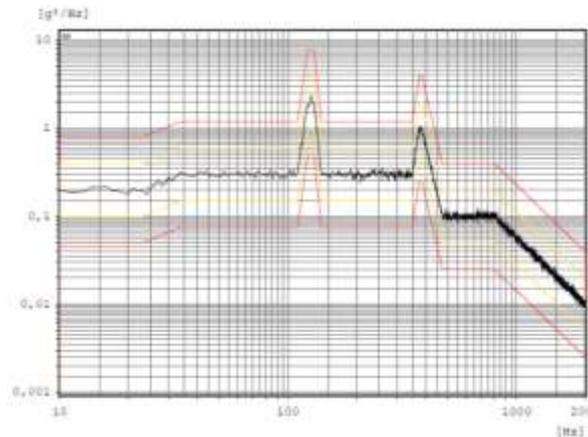
Figure 16: 16 g rms random vibration profile 16 g rms, Duration: 1 hour/axis, 3 axis
