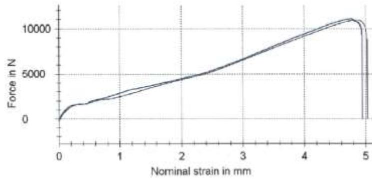
Figure 3. Tensile testing at 200 C
