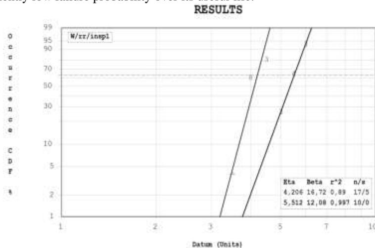
Figure 4. Weibull fit of fatigue failure amplitude for untreated (left-hand curve) and treated (right-hand curve) springs. Datum axis indicates stroke [mm].
