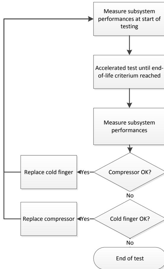
Figure 10. Test progression for accelerated testing with subsystem-level results evaluation.
