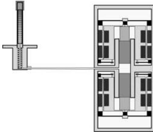
Figure 8. Schematic overview of Thales LSF cooler
