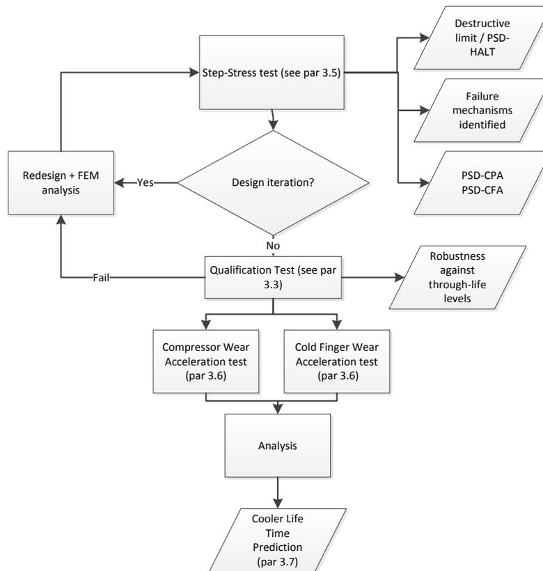
Figure 6. Overall test logic
