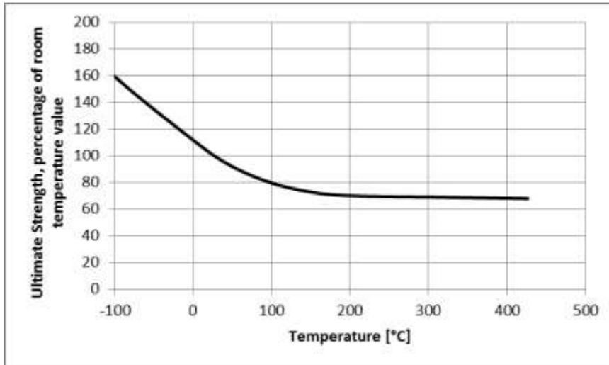
Figure 2. Ultimate strength vs temperature.
