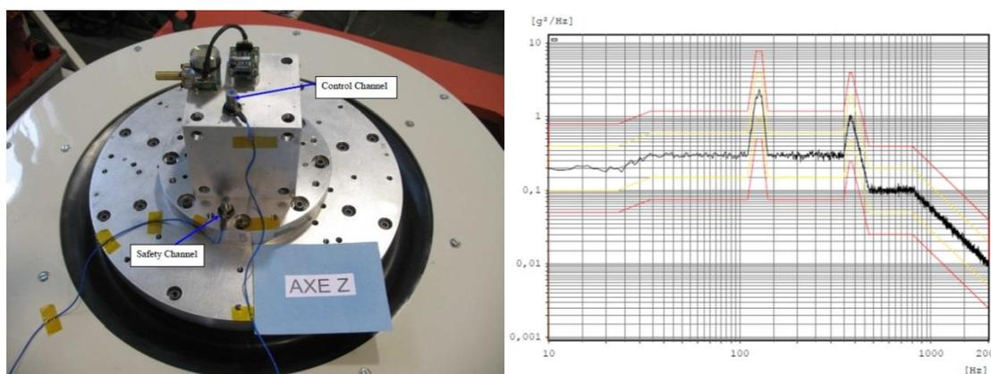
**Figure 11.** vibration test bench and 16 g rms random vibration profile 16 g rms,
