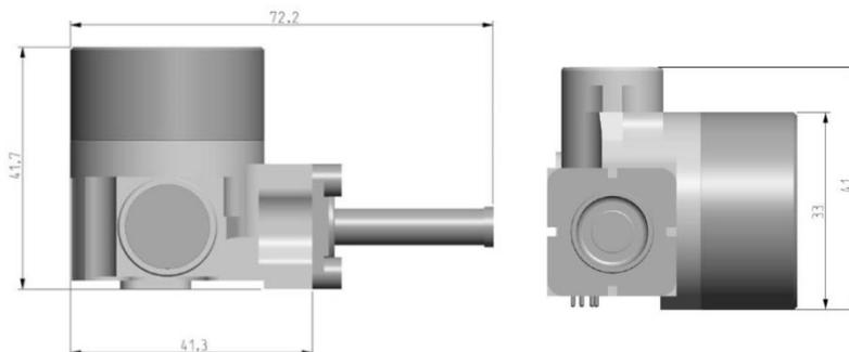
**Figure 1.** Overall dimensions of RMs1 integrated in common cold finger
