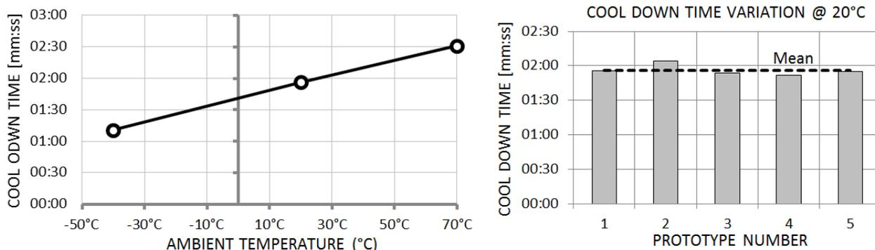
**Figure 3.** Cool down time as a function of ambient temperature (left), and variability of CDT between 5 units (right).
