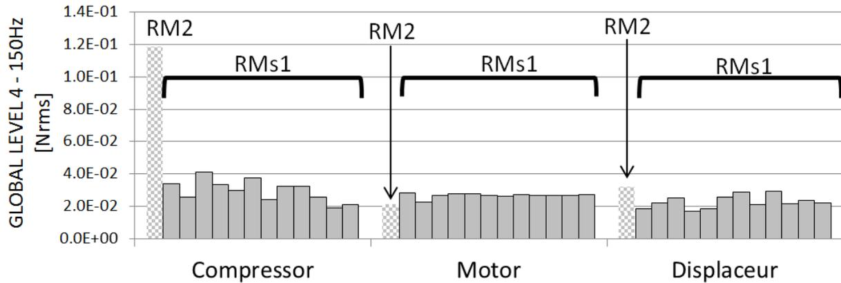
**Figure 9.** RMs1 global induced vibrations levels for 12 coolers between 4Hz and 150Hz and comparison with RM2
