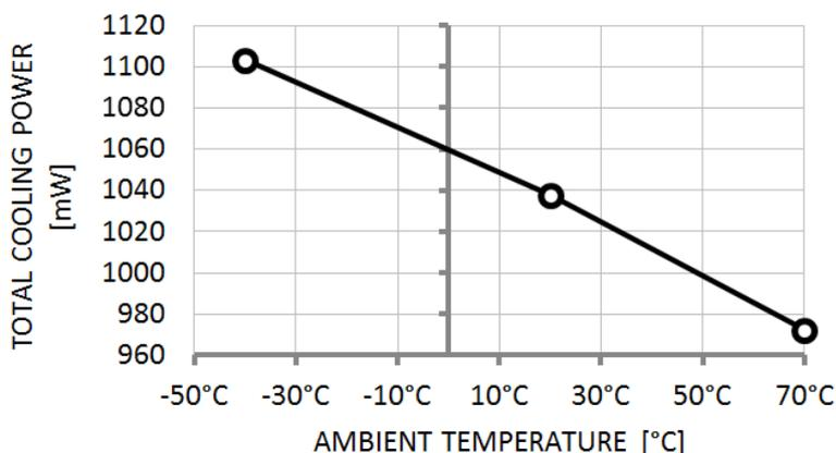
**Figure 6.** RMs1 total cooling power at 150K in function of ambient temperature
