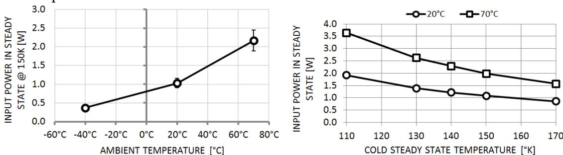
**Figure 4.** Steady state ac input power as a function of cold temperature and ambient temperature.
