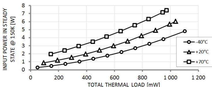
**Figure 5.** Steady state ac input power at 150K in function of ambient temperature and total cooling power.
