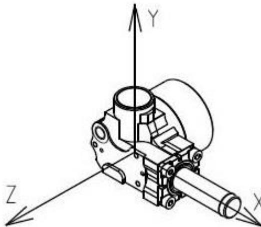
**Figure 8.** Induced vibrations axis
