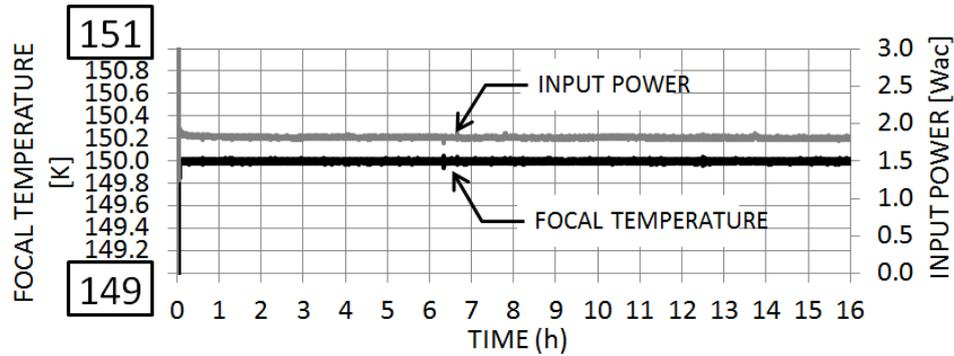
**Figure 7.** Temperature and input power stability during 16 hours at 70°C. the full scale is +/-1 Kelvin for focal temperature and 0-3W for input power.
